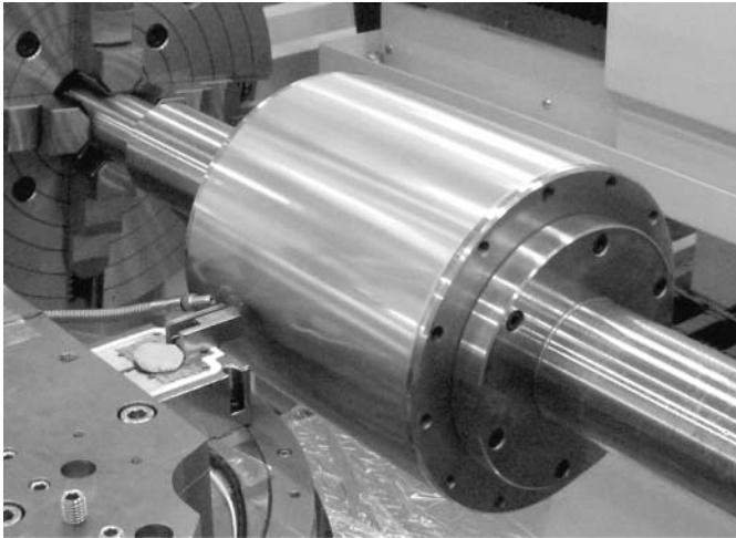
Figure 4.11 Dot pattern processing on the surface of a metallic roll
