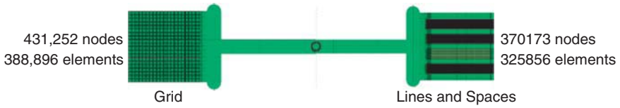
Figure 3.16 Mesh model of a molded product with micro-surface features of a grid and lines and spaces
